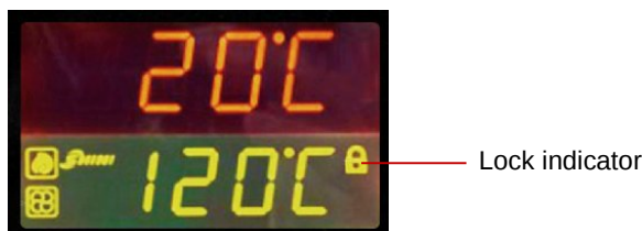
Picture 4-2: Temperature Lock
